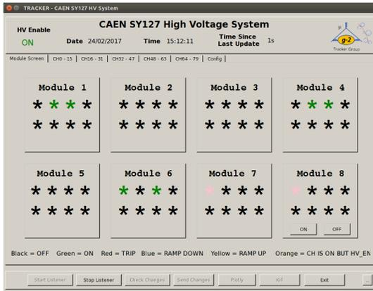
Figure 2. Main window of the Python GUI used to control CAEN SY127 power supply.
