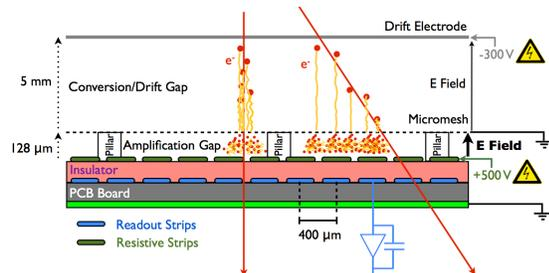
Figure 1. Bulk Micromegas with HV changes.
