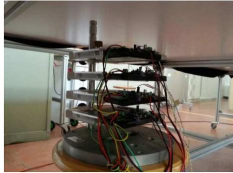
Figure 13. Small cosmic ray detector made by 4 scintillator tiles put into coincidence positioned under LUNA module.
