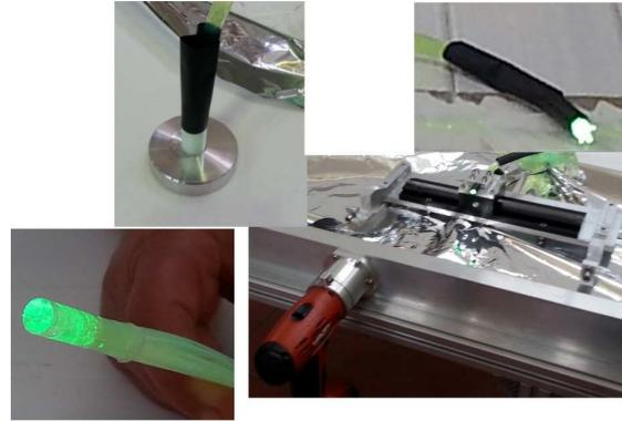
Figure 3. Sequence showing the bundle fiber polishing process.
