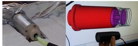
Figure 4. Mechanical structure for the PMT/fibers coupling and the correct positioning of the PMT inside the detector vessel together with the outer connection.
