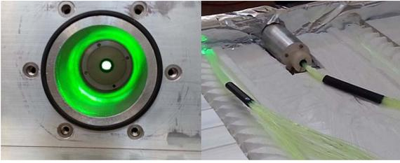
Figure 11. The Enclosure of the PMT
