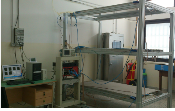
Figure 2. Picture of a MRPCs telescope station located in a Lecce's High School: Liceo Classico G. Palmieri .
