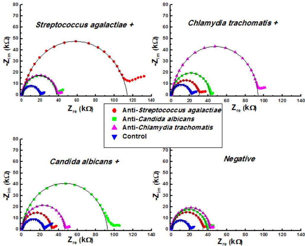
**Figure 2.** Nyquist plots for immunochips characterization with a sample containing *Streptococcus agalactiae* (A), *Candida albicans* (B), *Chlamydia trachomatis* (C) and without pathogens (D). Black lines are the fitting curve on the basis of equivalent circuit elements
