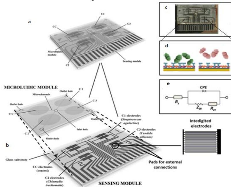
**Figure 1.** Scheme of the immuno-chip, including its components and equivalent circuit.
