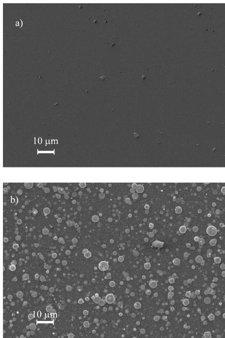
Figure 1. Plan-view SEM micrographs of (a) Y film and (b) Pb film on Si (100) substrates.
