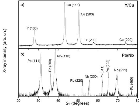
Figure 3.  $\theta - 2\theta$  XRD patterns of (a) Y film and (b) Pb film on Cu and Nb polycrystalline substrates, respectively.
