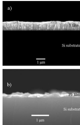
Figure 2. Cross sectional SEM images of (a) Y film and (b) Pb on Si (100) substrates. The Y and Pb thicknesses are about 1.2 μm and 300 nm, respectively.
