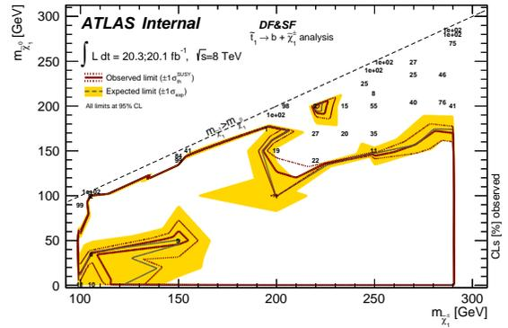
Figure 1. Exclusion limits at 95% CL in the  $m(\tilde{\chi}_1^\pm) - m(\chi_1^0)$  plane for a 300 GeV mass stop obtained from the combination of the MET trigger based and the Lepton trigger based analyses. The numbers shown in the plots are the observed CLs values.
