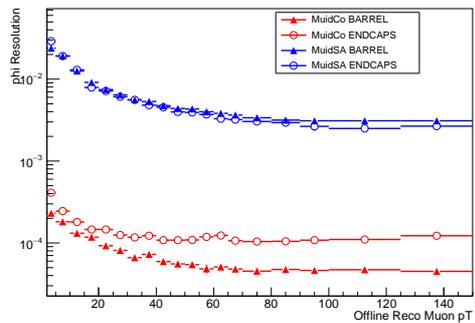
Figure 3. Spatial  $\varphi$  resolution with respect to offline as a function of muon offline transverse momentum.
