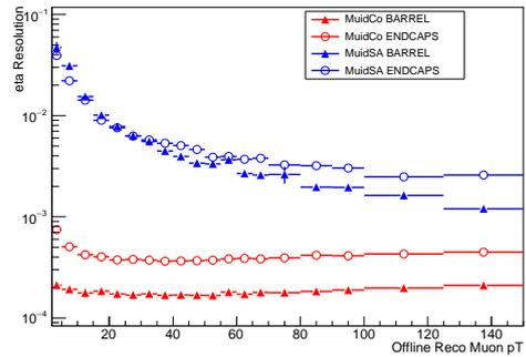
Figure 2. Spatial  $\eta$  resolution with respect to offline as a function of muon offline transverse momentum.
