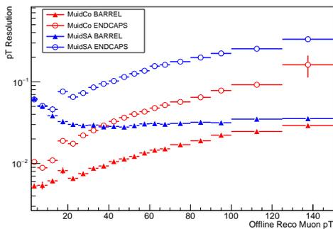
Figure 1. Transverse momentum resolution with respect to offline as a function of  $p_T$  for MuidCo and MuidSA algorithms, separately for barrel and endcap regions.
