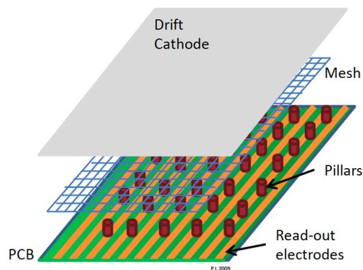
Figure 1. MicroMegas chamber layout.
