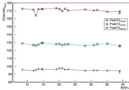
Figure 6. Behaviour of the peak position as function of the T1 gas relative humidity for different read-out voltages applied to T2.
