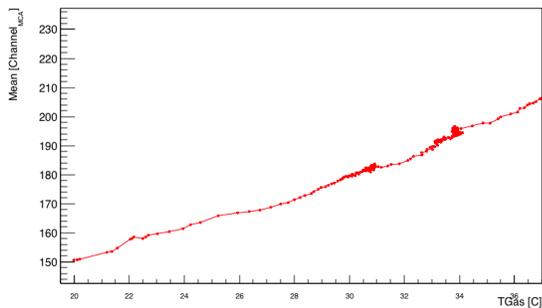
Figure 7. Behaviour of the peak position as function of the T5 gas temperature.
