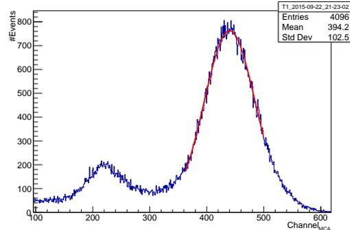
Figure 4. <sup>55</sup>Fe spectrum in MultiChannel Analyser unit obtained from a gas mixture of Ar:CO<sub>2</sub> (93:7). For each measure the main peak has been fitted by a gaussian and the gaussian mean has been assumed as peak position.
