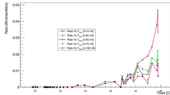
Figure 9. Sparks rate as function of the T1 gas temperature for different current threshold.
