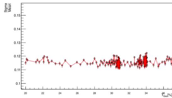
Figure 8. Behaviour of the resolution as function of the T5 gas temperature.
