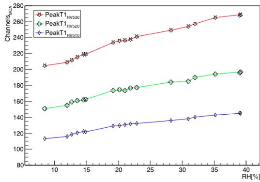
Figure 5. Behaviour of the peak position as function of the T1 gas relative humidity for different read-out voltages applied to T1.
