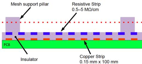
Figure 3. Sketch of the layout of a bulk MM detector.
