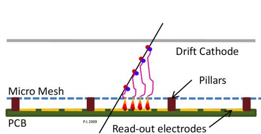
Figure 2. Schema of MM operating principle. The electrons produced into the drift area drift to the amplification region where the avalanche will be produced.
