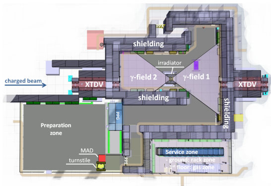
Figure 2. GIF++ bunker layout. An energetic beam of charged particle (mainly muons) is overlapped to a photon flux of 662 KeV produced by ^{137}\text{Cs} source of 13.9TBq. A filter system is also present to attenuate the photon rate. All the information about ambient variables, beam and source status, attenuation used are provided by DIP system.
