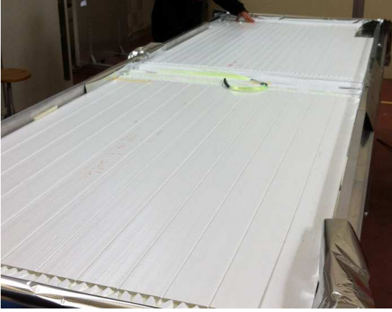
Figure 2. Complete view of the two module, LUNA and TERRA, before closing the detector.
