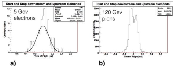
Figure 2. Distribution of the time-of-flight between two polycrystalline diamond detectors placed parallel to a 5 GeV electron beam, after correcting for track entrance point vertical dependency (a), and placed parallel to a 120 GeV pion beam (b). The high voltage value was -350 V and 500V, respectively.
