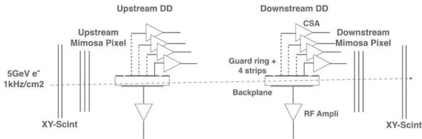
Figure 1. Experimental setup used to measure the time-of-flight between two diamond detectors placed parallel to a 5 GeV electron beam at DESY. A similar setup was used in a testbeam with 120 GeV pion beam at CERN.
