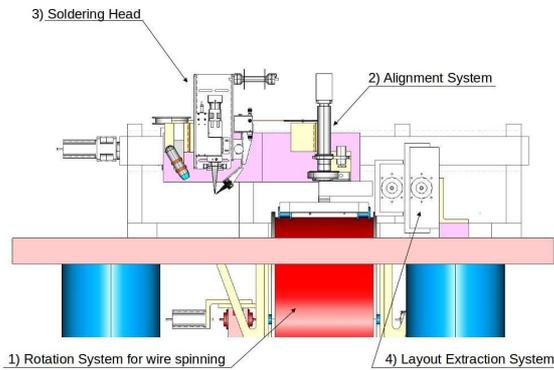
Figure 2. Schematic view of the wiring system.
