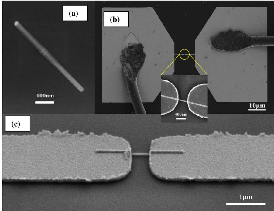
**Figure 1.** SEM images of (a)  $45 \pm 10$  nm diameter InAs/InP nanowires with a QD region defined as a 20 nm long InAs island sandwiched between two epitaxial 5 nm-thick InP barriers; (b) contact pads and nanoelectrodes; (c) a typical InAs/InP heterostructured nanowire deposited on a SiO<sub>2</sub>/Si substrate and contacted by two Au/Cr electrodes.
