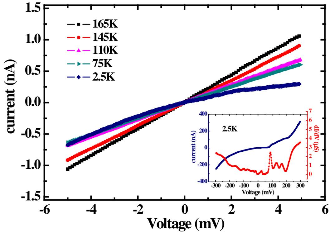
*Figure 2. I-V characteristics and temperature dependence of a nanowire junction. The inset shows the I-V curve (blue line) and the measured  $dI/dV$  spectrum (red line) at low temperature (2.5 K).*
