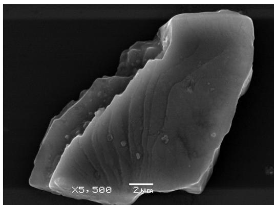
Figure 2. SEM image of particles of the calcite mineral.
