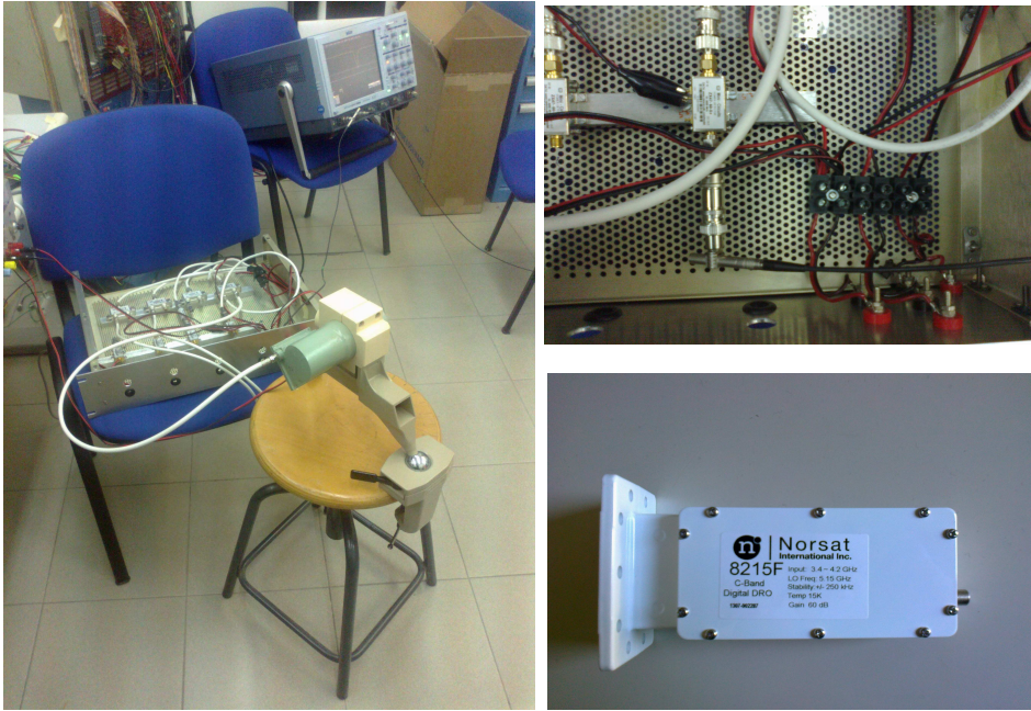
Figure 2. Experimental setup for feed characterization including the electronics box and the oscilloscope (left). Shows in figure is also the power detector (right top) and the LNB chosen for the construction of the prototype (right bottom).
