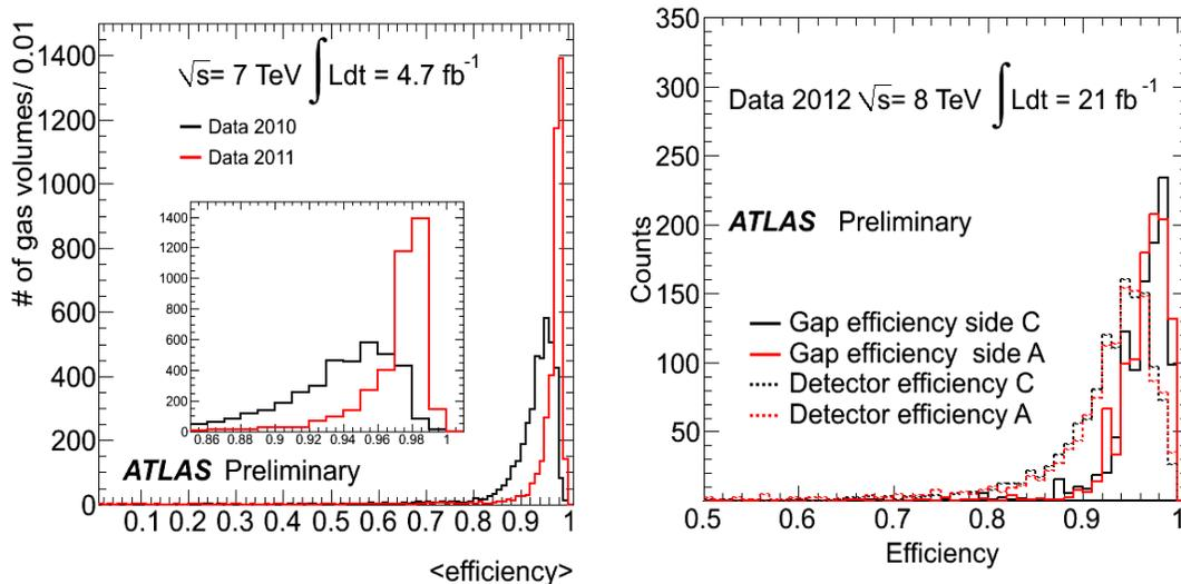
Figure 1. Distribution of the RPC gas volume efficiencies measured in 2010, 2011 (left) and 2012 (right) data taking periods. The gas volume efficiency are separated in side A and side C for the right plot.
