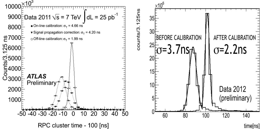
Figure 2. The plots show the distribution of RPC time in readout hits for both views before and after offline calibration in 2011 (left) and 2012 (right) data taking periods. The time of the hits is shifted of 100 ns in the left plot.
