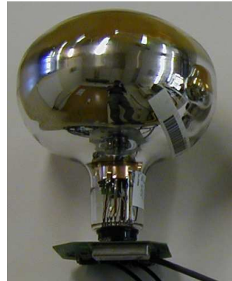
Figure 1. A picture of the PHOTONIS Photomultiplier Tube (XP1805) connected to the High Voltage electronic card.
