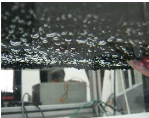
Figure 6. Air bubbles remaining below the black top layer after a freezing/unfreezing cycle.
