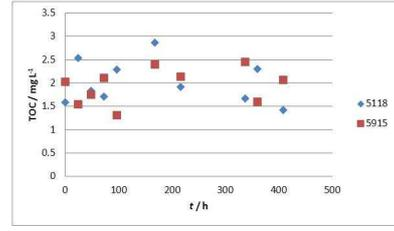
Figure 4. TOC in Water with spheres 5118 at 80 Celsius. 400 h = 17 days.
