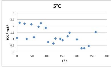
Figure 3. TOC in Water with spheres 5118 at 5 Celsius. 350 hr = 15 days.
