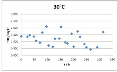
Figure 2. TOC in Water with spheres 5118 at 30 Celsius. 350 hr = 15 days.
