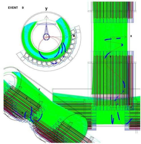
Figure 2. Simulation of a  $52.8\text{ MeV}/c$  positron track in the new drift chamber.
