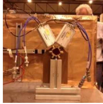
Figure 3. Diamond detectors connected to Front-end electronics in experimental area during the October 2012 testbeam at T4-H6 North Area CERN with 120 GeV pion beam.
