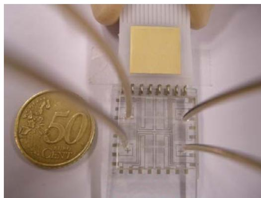
*Figure 1. Biochip layout with interdigitated electrodes, temperature sensors and heaters, PDMS microfluidic components (chambers with microchannels), inlet and outlet tubes.*
